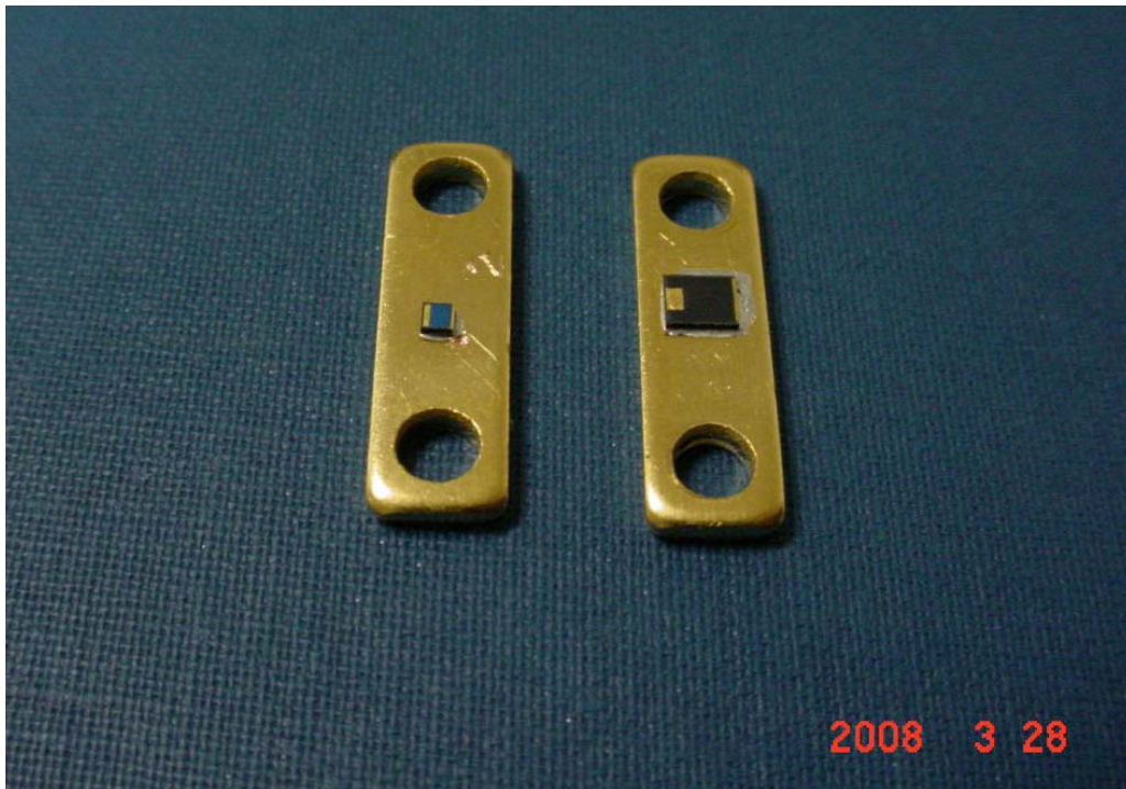
CT0505D & CT1310D Soldered to Gold Plated Copper Flange.
